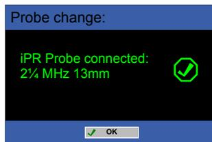
The selected probe will then be displayed at the bottom right of the screen in measurement mode.
