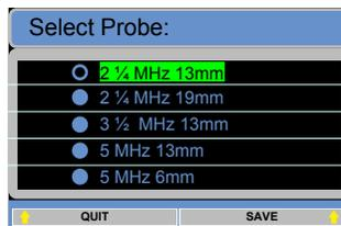
Press 'Option Key 2' (6) to save the selection. The selected probe will be displayed at the bottom of the screen in measurement mode.
