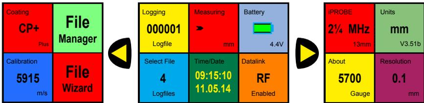
**Coating Plus+** - Allows measurements to be taken through extremely thick coatings up to 20mm, depending on the type of coating. In normal mode the gauge can still ignore up to 6mm of coating.
