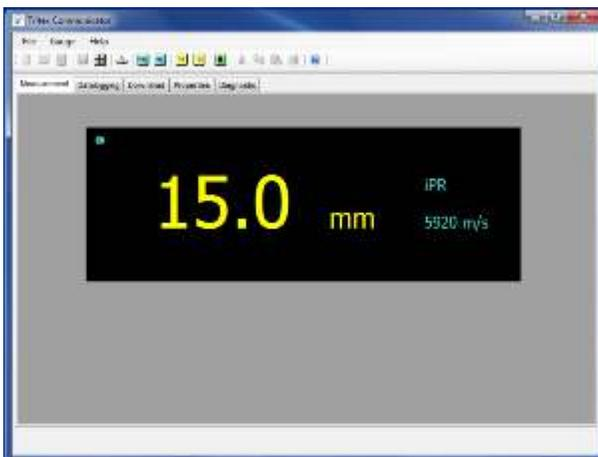
The *Measurement tab* is used to view measurements received from the gauge in the simplest form, with large scale digits for convenience.
