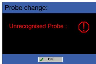
This is a prompt to select the correct setting for the probe that has been connected. Press 'OK' (4) and then use the 'Up' (5) and 'Down' (9) arrow buttons to select from the following displayed list:
