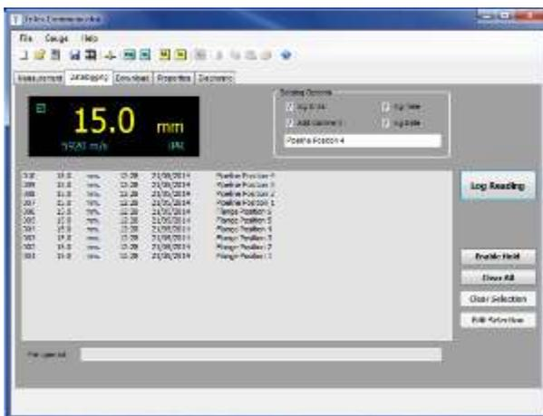
Measurements are added to the list by clicking on the
