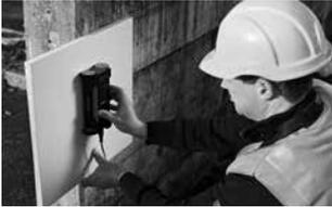
For correct cover measurements the sheet thickness must be set as Cover Offset value.
