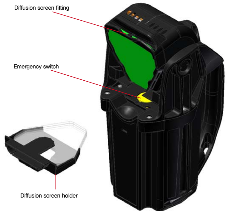
Fig. 5 (emergency switch and diffusion screens)
