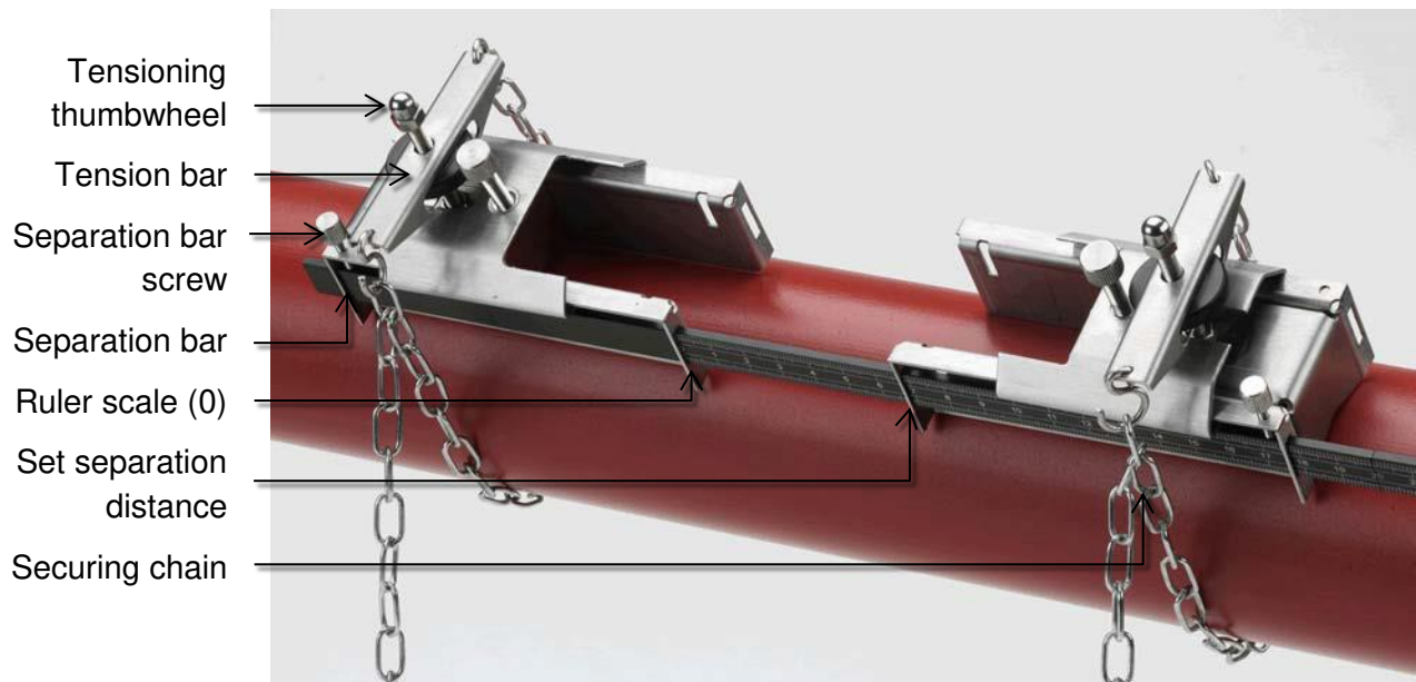
Figure 8 Guide rail assembly
