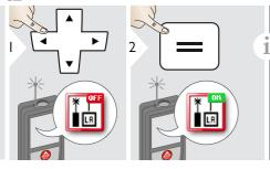
The long range mode allows measuring of difficult targets in unfavorable conditions e.g. bright ambient light or bad target reflectivity. The measuring time is increased. An icon in the status line shows if the function is active.
