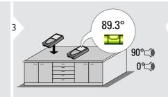
Inclination is permanently displayed. Instrument beeps at 0° and 90°. Ideal for horizontal or vertical adjustments.
