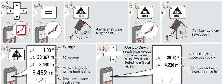
Indirect distance measuring between 2 points with additional results. Ideal for applications such as length and slope of roof, height of chimneys,... It is important, that the instrument is positioned in the same vertical plane at the 2
