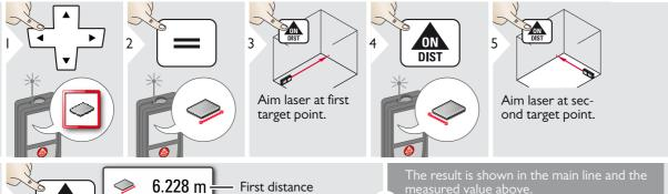
Partial Measurements / Painter function: Press + or - before starting the first measurement. Measure and add or subtract distances. Finish with =. Measure 2nd length.
