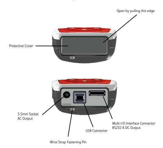
The **optimus** can be powered via the multi-pin connector on the bottom of the instrument. Power can be connected using a ZL:171 **optimus** power input cable (2.1mm Power Jack, 2m) or via ZL:176 **optimus** 12v Battery pack cable.
