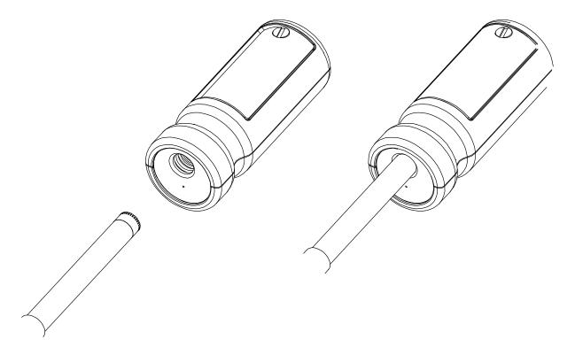
Ensure that the small bleed hole next to the microphone cavity on the calibrator is not blocked, as this could cause damage to the microphone.
