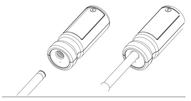
The microphone should be parallel to the body of the calibrator. Also ensure that the small bleed-hole next to the microphone cavity is not blocked as this could cause damage to the microphone.
