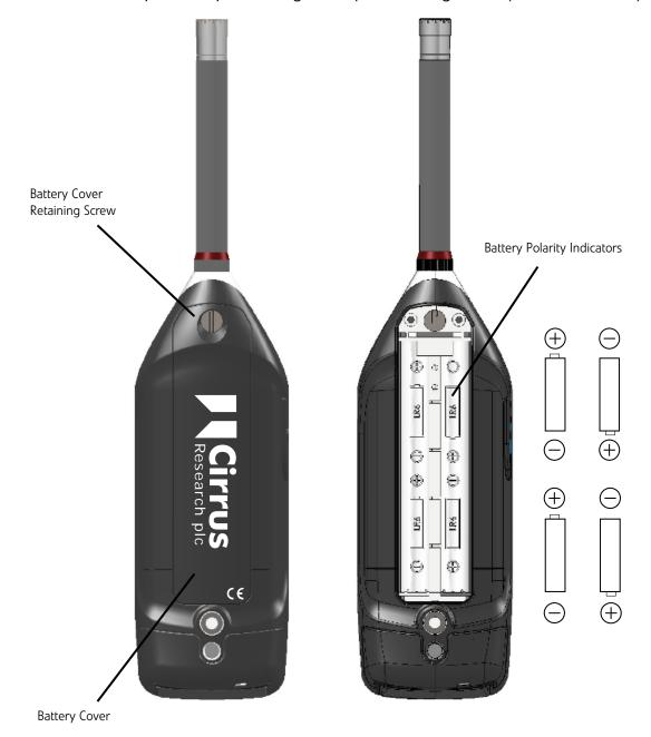
Please look carefully at the diagram inside the battery compartment showing the correct polarity. After inserting the batteries in the correct orientation, replace the cover and tighten the locking screw.
