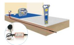
**Live cable connectors (Optional)** For applying the transmitter signal to a live cable, the most certain method of locating a power distribution system in a street.
