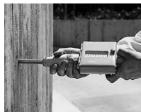
Fig. 2.2 Deploying the impact plunger (1) (model NR)
