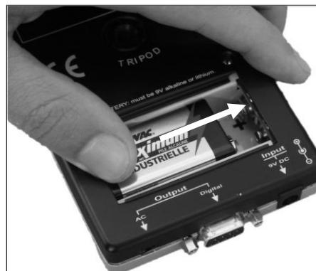
When this icon appears, the SC160 battery must be replaced. The SC160 will show the symbol for 5 minutes (if a measurement or a recording is in progress). Then it will stop measuring, the “BATTERY FLAT” message will appear on the screen and then the SC160 will automatically switch itself off. Do not use rechargeable batteries, nor attempt to recharge the flat battery.
