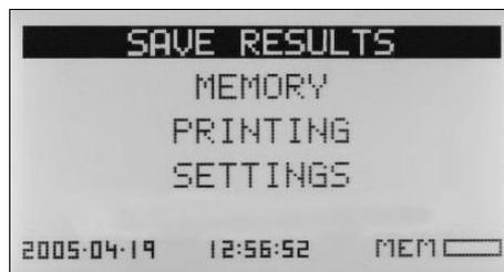
This screen shows the main settings menu together with the date and time on the SC160 clock. Information is also available on the state of the memory, indicating the amount of memory occupied.
