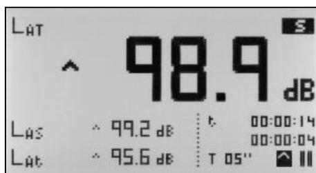
When **over** appears in the indication of the value of a function, this means that the value measured exceeds the upper limit of the measurement range (over-range). When this happens, the maximum range of the SC160 has been exceeded and the current level cannot be known, thus any such measurements should be discarded.
