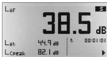
The frequency weighting displayed for the three functions is changed by pressing
